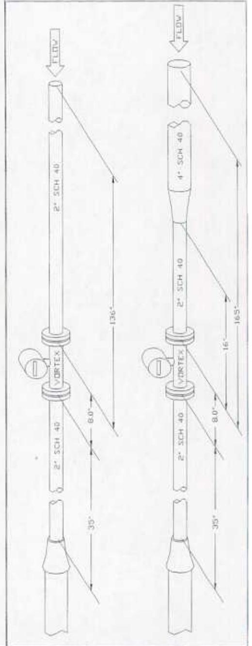
AS FOUND STRAIGHT RUN AND REDUCTION WITH VORTAB (IN AIR) - Figure 16
