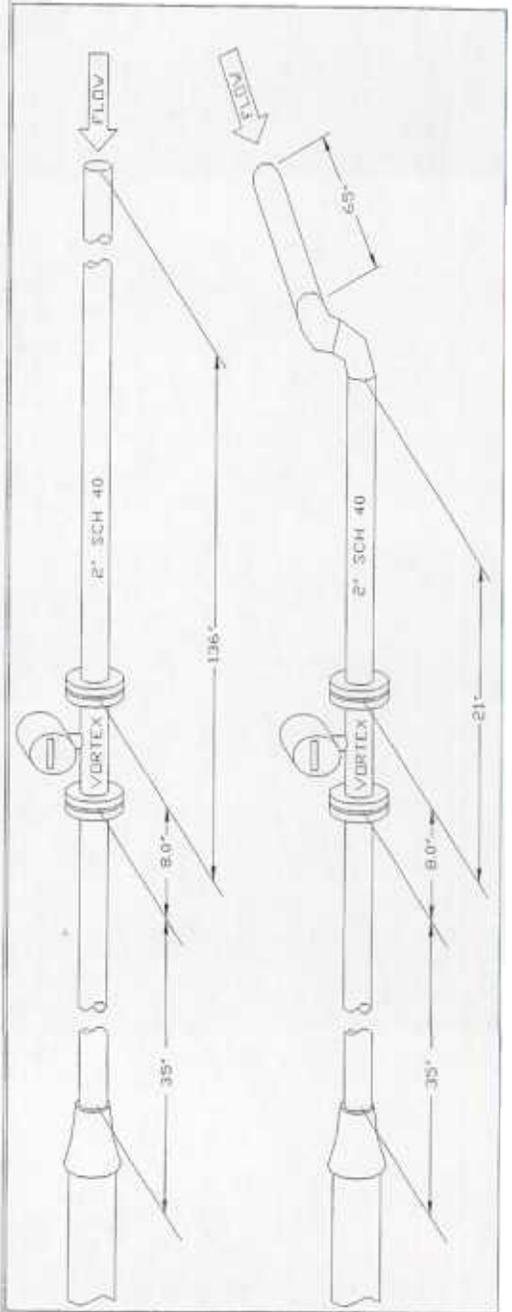
**AS FOUND STRAIGHT RUN AND 2 OUT OF PLANE ELBOWS WITH VORTAB (IN AIR) - Figure 20**
