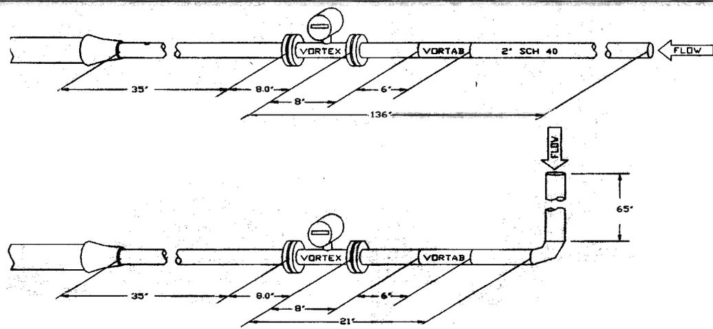
AS FOUND STRAIGHT RUN AND 2 OUT OF PLANE ELBOWS WITHOUT VORTAB (IN AIR) - Figure 19
